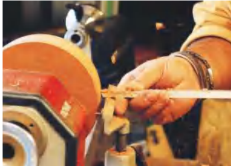
▲ Each tool addresses the work at around 90° to make the cut
